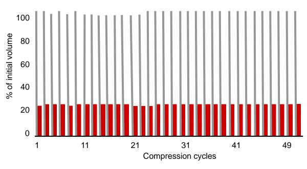
In vitro compression test shows volume maintenance upon repeated compression of the hydrated matrix<sup>1</sup>. Gray bars represent the regained/ initial volume of the matrix; red bars show the compressed volume.
