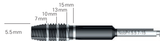
37997 Screw Tap NobelParallel CC Ø 5.5 7–15 mm
