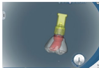
After scanning the wax-up (using the NobelProcera 2G Scanner), a molar crown is designed using the NobelProcera software.
